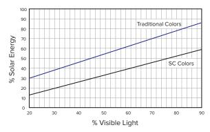
**Note:** Both Polycast UV-SC materials transmit high amounts of visible light (400 to 700 mm) and transmit much less radiation in the near-infrared (NIR) and in the UV. The NIR and UV regions contain significant amounts of solar energy, but do not contribute to visibility.
